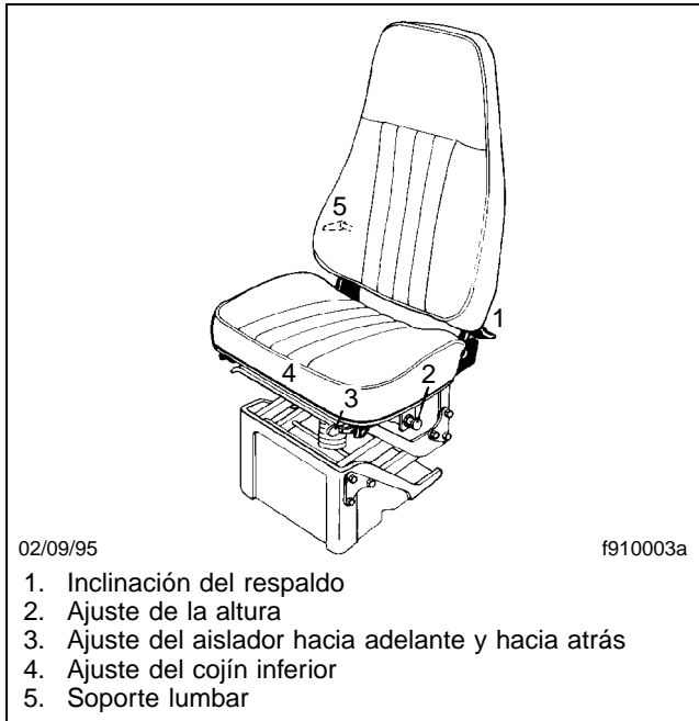
Figura 5.3, Asiento Fleetcruiser Dura-Form
